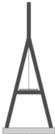
Fig.14. Three Plane Pylon front view.
