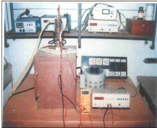
Fig.8 Instrument of Parallel to c-axis resistivity measurement Fig.9 Schematic diagram of the Instrument
