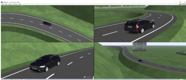
Figure 4.5 Different view of our model in IPG Movie We have to set the coefficient of friction for the road. We had taken the dry asphalt road (the co-efficient of friction is 0.4) as shown in Fig. 4.6.
