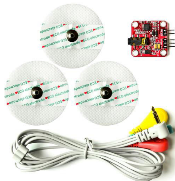
Figure 1. Surface EMG setup
