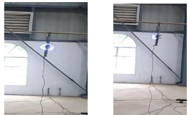
Fig. 9 Flashover of (a) straight shed Insulator (b) alternate shed insulator
