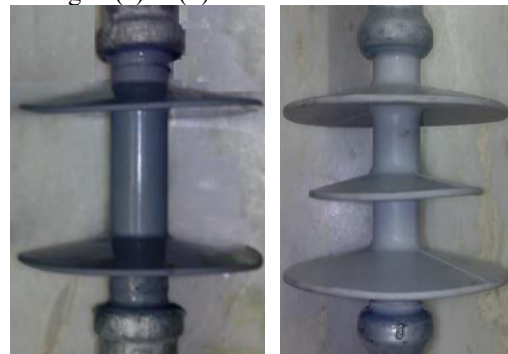
(a) Straight shed (b) Alternate shed Fig. 4 polymeric insulators
