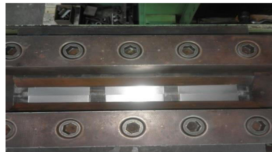
Fig – 2: Plates in clamped position in FSW machine
