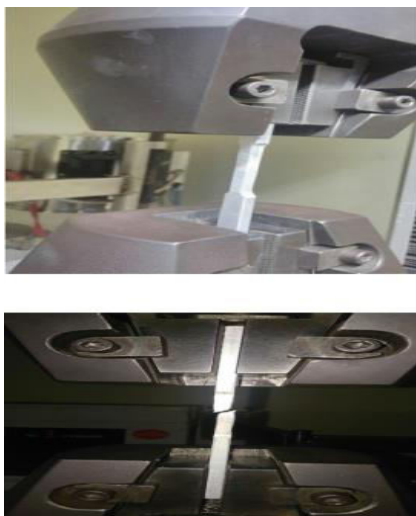
Figure. 3 : Tensile test conducted in UTM
