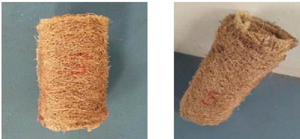
FIG. 9: Luffa-Cylindrica or Sponge Gourd vegetable fiber Stitched to Cylindrical core as reinforcing material
