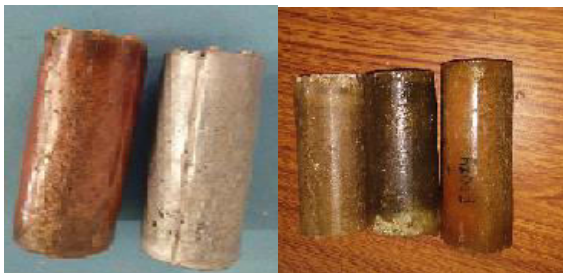
FIG. 10: Fabricated cylindrical Polymer Matrix Composite samples with required diameters
