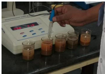
Fig. 3. Measuring Soil pH
