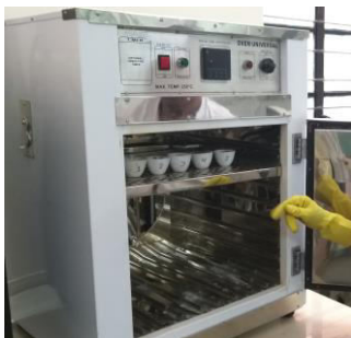
Fig. 4. Measuring Soil Moisture Content in Hot Air Oven
