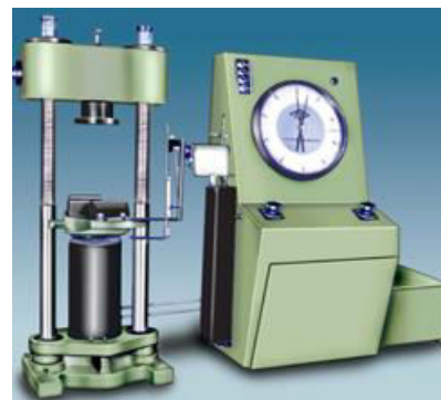
Figure 4.12 Universal Test M machine (for flexural test & tensile test)
