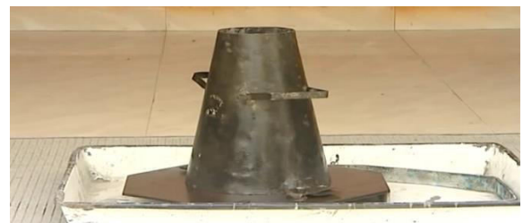
Fig 3.2.1 Concrete Filling in Cone
