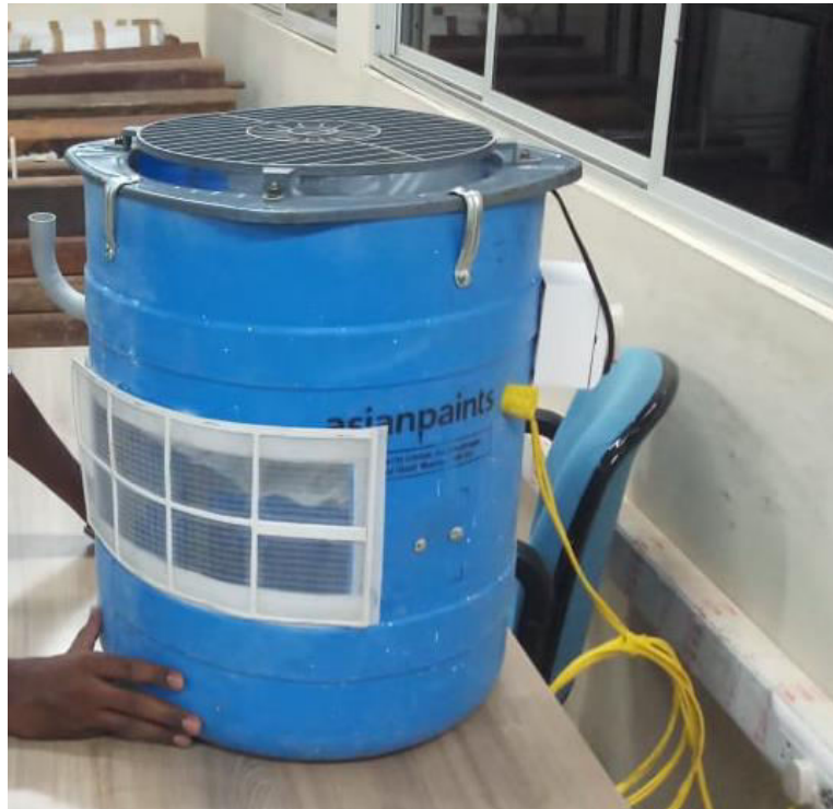
Fig. 8. Fabricated Cooling tower
