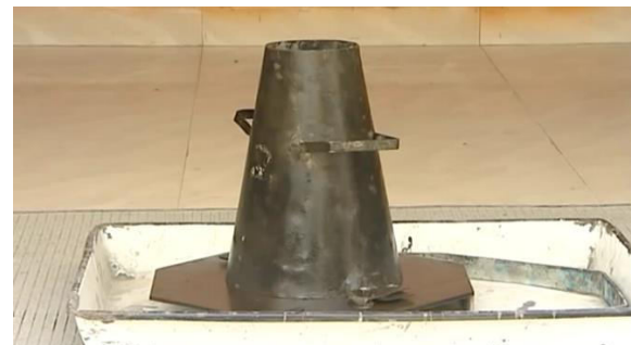
Figure 7.1 Concrete Filling in Cone
