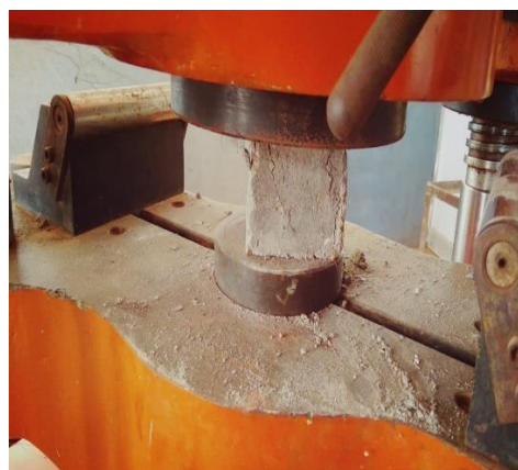
Fig: 7.1 Cube tested in UTM machine
