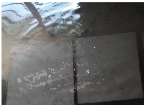
Fig 6.1: Tiles immersed in water for water absorption test
