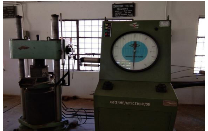
Figure 4: compressive strength test on cube
