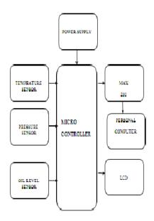
PIC is used to connecting the device and sensors .Sensed instruction given to PIC controller and control on the WANET for
