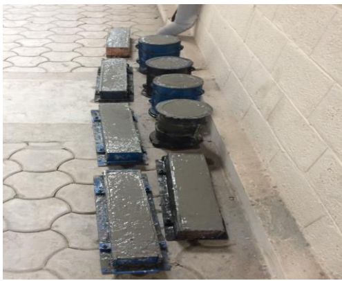
Fig 1: Moulds filled with concrete
