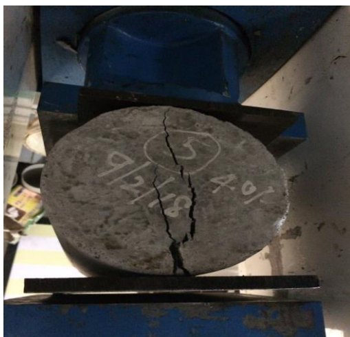
Fig 3: Split Tensile Strength Test
