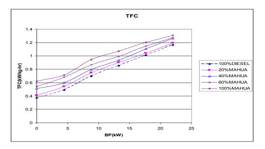
It can be observed from the graph, as the brake power increases the TFC is increasing. But diesel has the least of all the other biodiesel blend when compared.
