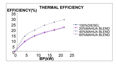
It is noted from the graph, as the brake power increases, combustion efficiency increases. The delay period decrease with increasing load because the operating temperature of the engine increases, leading to better combustion.
