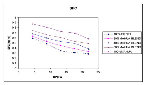
It can be noted from the graph, the SFC decreases with an increase in brake power. It is also absorbed from the graph that SFC for diesel is the least of all other Esterified mahua oil blends. It is because the lower calorific value will lead to increase in specific fuel consumption.
