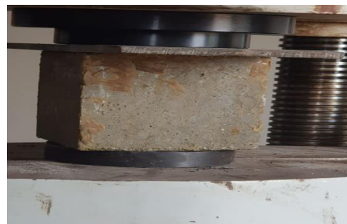
Fig.2 Concrete Compression testing Flexural strength of concrete
