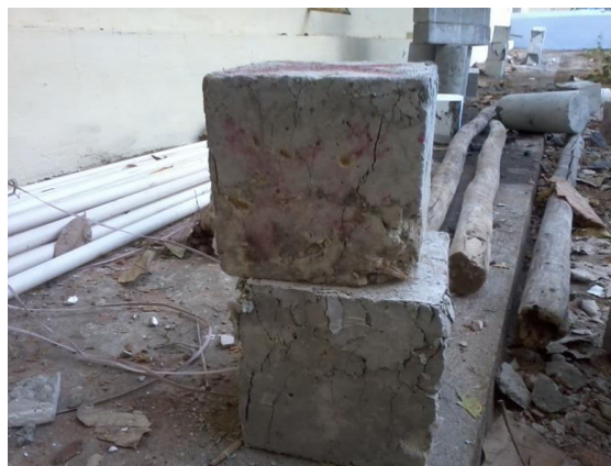
Failure of cube
