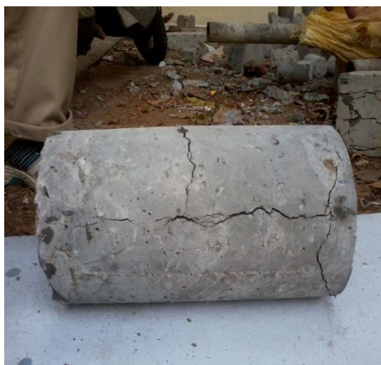
Failure of cylinder
