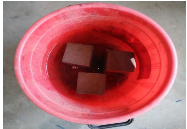
Figure. Water absorption test
