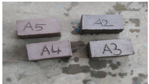
Figure. Casted bricks (Trail 1)
