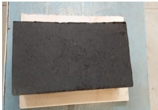
Fig 8 Bagasse Ash Bricks after De-moulding
