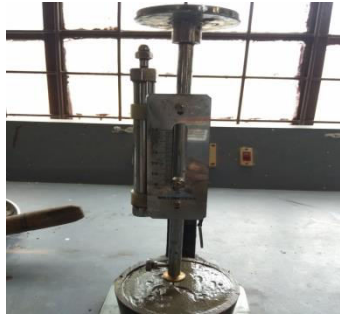
Figure 14: consistency test for cement
