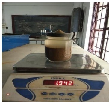
Figure 11: Specific gravity test for fine aggregate
