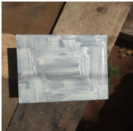
Figure 16: Coating with primer
