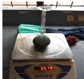
Figure 12: specific gravity test for cement
