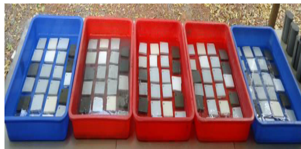
Fig. 5 Specimens immersed in different Chemical solutions
