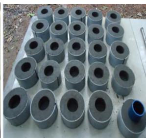
Fig. 2 Finished Hollow core Specimens
