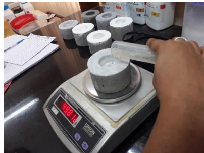
Fig 5. Water absorption test for hollow core specimen
