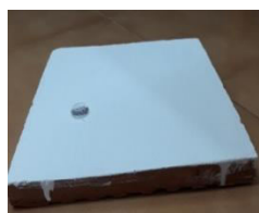
Fig. 3 Water Droplet on coated surface of roof tile
