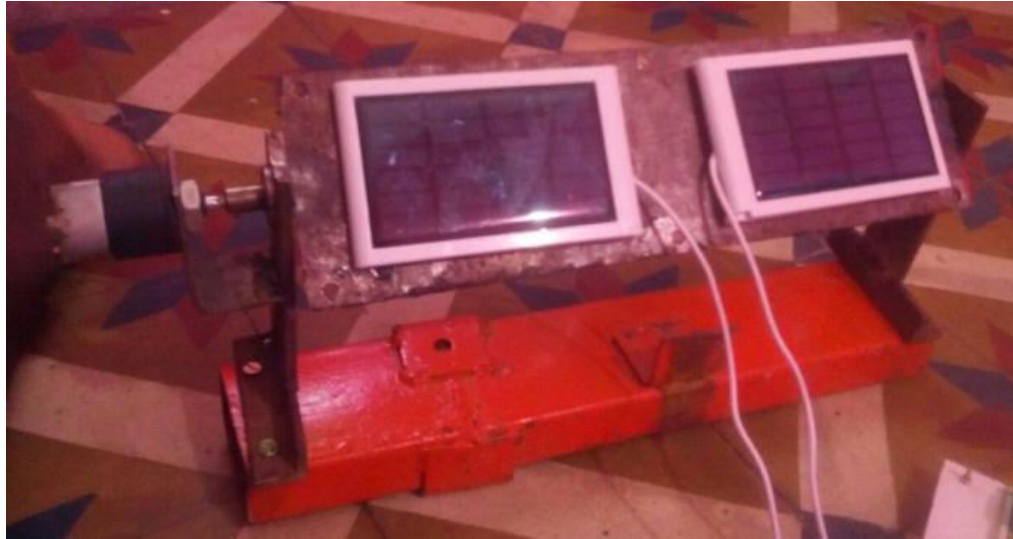
Fig. 6 Solar Tracking Setup
