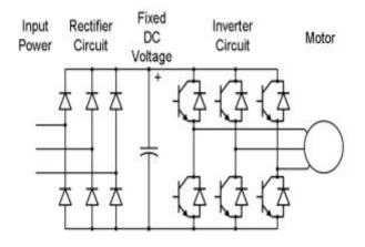
Variable frequency drives (VFD's) are often recommended as a way to save pumping energy. Actual energy savings will vary greatly depending on how the discharge pressure of the constant speed pump is controlled and how it is operated after the VFD is installed [12]. The speed of the motor can be changed by various methods such as hydraulic or eddy current coupling, variable pulley, gear box system etc.,
