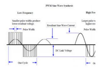
but most efficient one method is change the supply frequency and voltage to the motor. The variable frequency drive (VFD) varies the frequency and hence varies the speed of the motor as per the requirements by the load [13].
