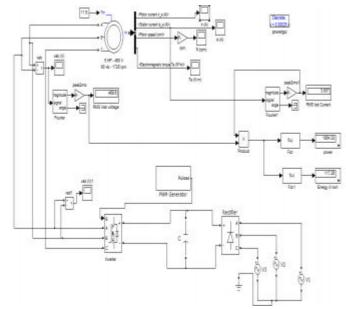
Speed control of AC/DC motors can be achieved by the variable speed drive (VSD) unit as shown in fig.2.1.
