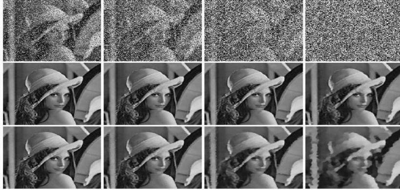
Fig. 1. Lena image blurred with out-of-focus kernel of radius 3, and then corrupted by salt-and-pepper noise with noise levels 30%, 50%, 70%, and 90% respectively.
