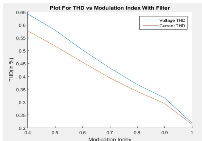
Fig. 21. Graph of THD Vs modulation index without filter with filter.
