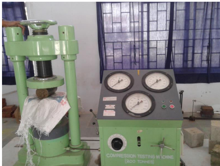
Fig. 4 Concrete cylinder Testing Arrangement
