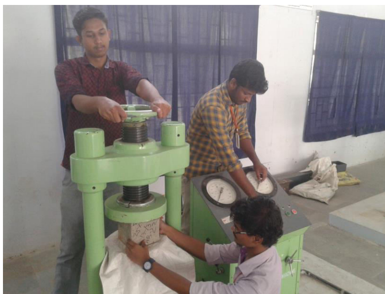
Fig. 2 cube Testing Arrangement
