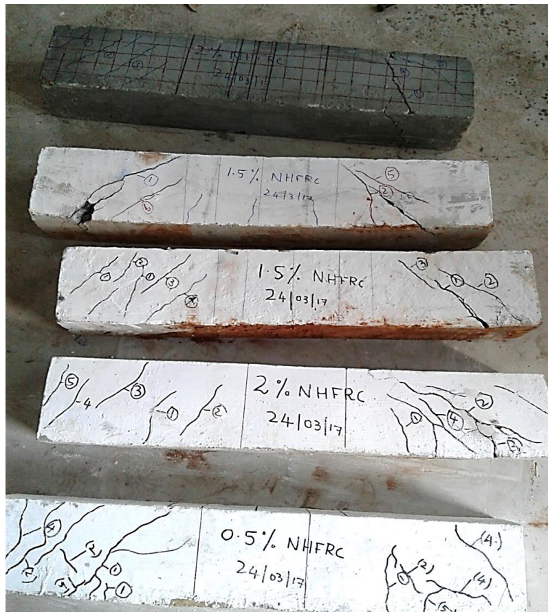
Fig.10. Beam specimens after testing with various percentage of NC & NHFRC
