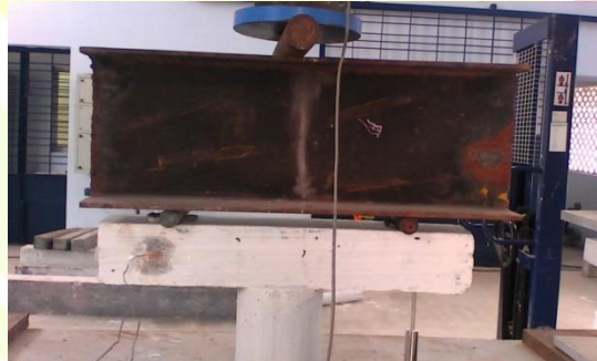
Fig 6: Model Testing for Deflection
