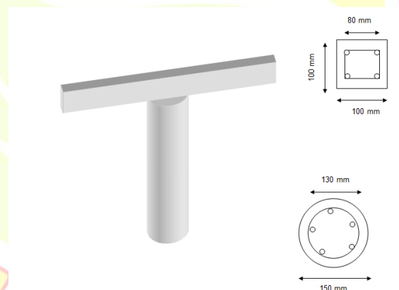
DETAILING OF BRIDGE MODEL
