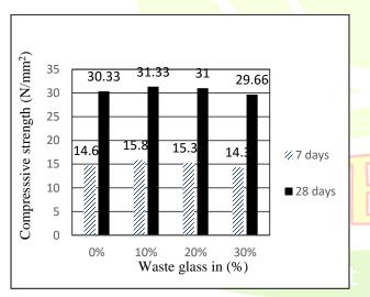
Fig.2- Variation of Compressive Strength of cubes
