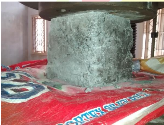
Fig 5.1 Compressive Strength Test on concrete
