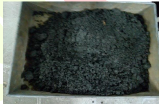
Fig 4.2.1 Wet mix of coarse aggregate, cement, FLP, Quarry dust, Iron slag
