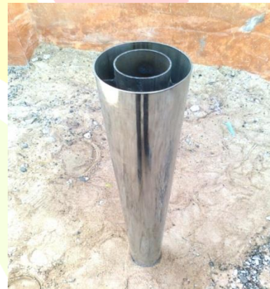
Fig 4.4 Photographic view of CFDSCT before casting.
