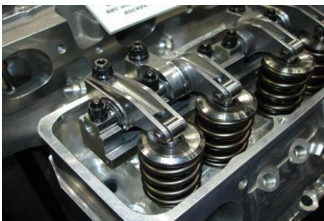
Fig. 1. Rocker Arm Assembly [9]
