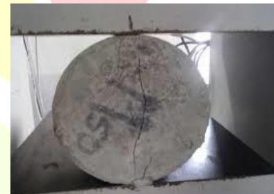
Figure 3. Testing of Cylinder
