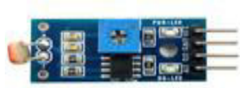
Fig.5. Room Light Sensor
