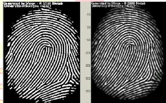
Fig. 8 the Fingerprint image after adaptive binarization Binarized image(left), Enhanced gray image(right)
