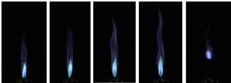
Fig. 2 Flame images at equivalence ratio \phi = 1.86 and lift off velocity = 2.48 m/s
