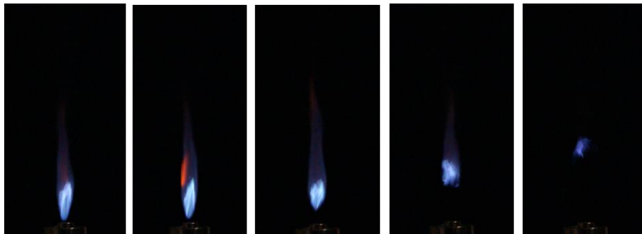
Fig. 3 Flame images at Equivalence ratio \phi = 1.2 and lift off velocity = 3.2 m/s
