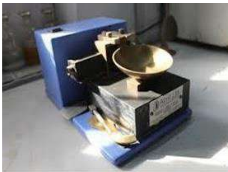
Fig 7.3 Casagrande liquid limit apparatus
