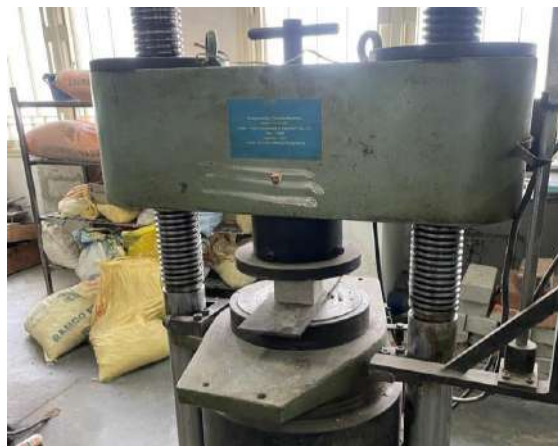
Fig 6.2 Compressive testing of metakaolin incorporated cube
