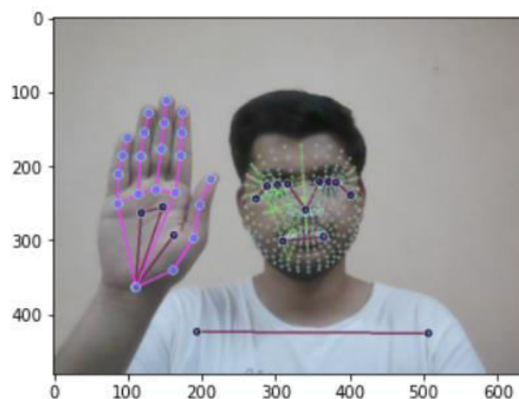
Fig. 3. Keypoint detection using mediapipe Holistic
