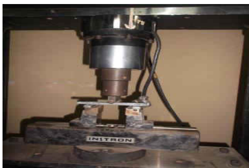
Fig 5.2 Three point bend test loading arrangement
