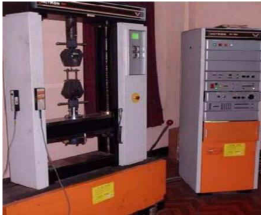
Fig 5.1 Experimental set up for tensile test
