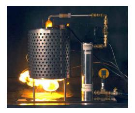
Limited testing ("Dust Screen") can also be performed by way of screening at predetermined temperature values to address specific process situations and needs. The equipment and ignition criteria remain identical to that of the full method described above.
