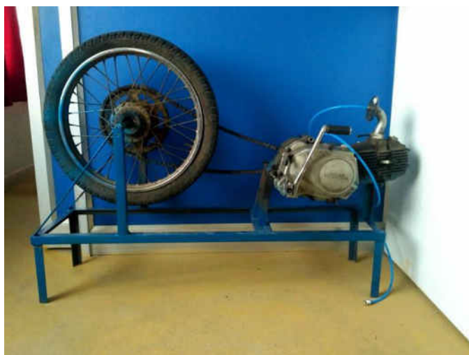
Fig 3: Prototype of compressed air-engine
