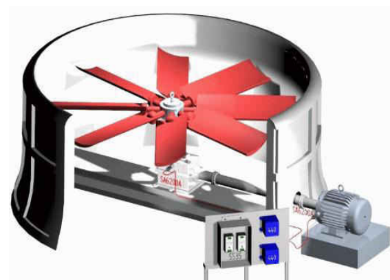
Fig.2 Induced Draft Fan Motor with VFD
