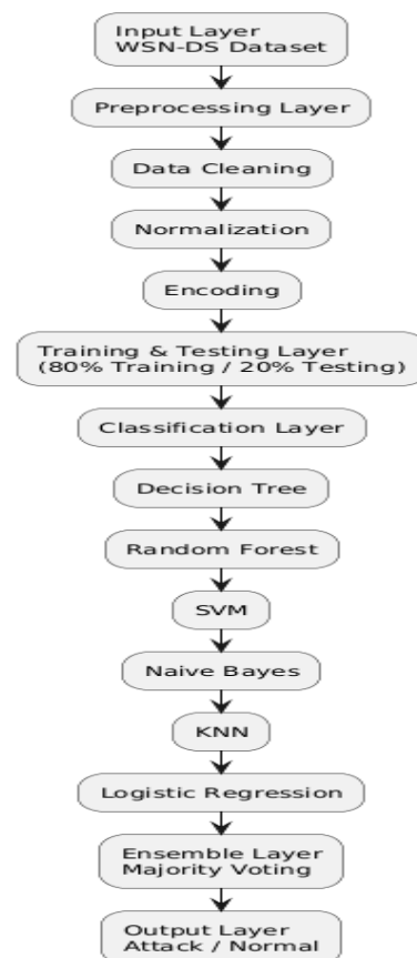
Fig 3.1. Machine learning pipeline for intrusion detection using the WSN-DS dataset.
