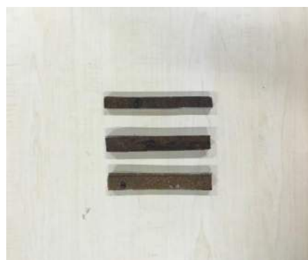
Figure-4 Flexural test specimen
