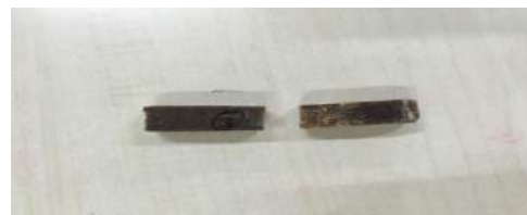
Figure-12 Flexural after test specimen
