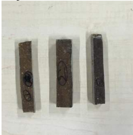
Figure-5 Charpy test specimen
