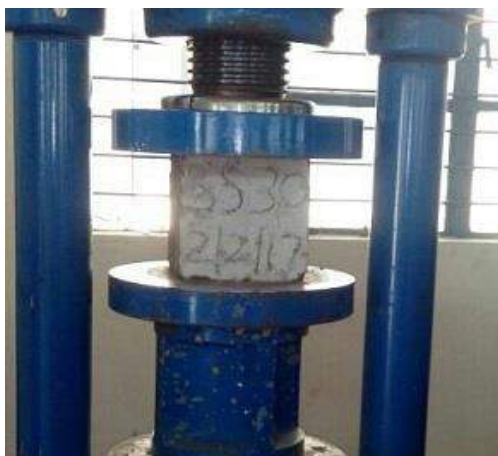
Fig 4.1 Compressive Strength Test
