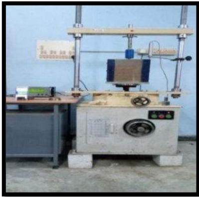
Fig 3 : Plate load test setup
